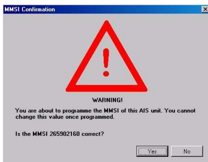
Figure 17 Before AIS-CTRX CARBON be programmed, this warning will always appear to ensure that the correct MMSI numbers have been entered.
