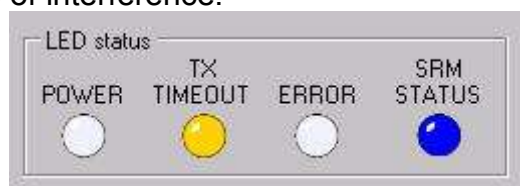
Figure 23 The blue LED will shine when AIS-CTRX CARBON is set to function only as an AIS receiver, "SILENT MODE".
