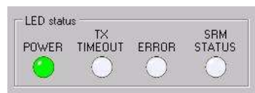
Figure 24 The green LED means that everything is OK.
