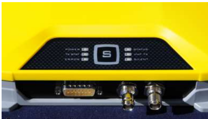
Figure 8 AIS-CTR X CARBON connectors. From the left the 15 pole d-sub connection (Male) for data and DC power supply, TNC (Female) for GPS antenna, BNC (Female) for VHF antenna (a BNC to UHF adapter is provided if required). We do however recommend to use a BNC connector direct on the VHF antenna cable.
